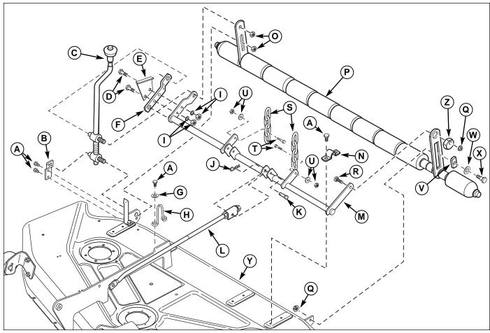
Figure 3. Install 54" Roller Bar A. Capscrews, 5/16-18 x 3/4 (Existing)
